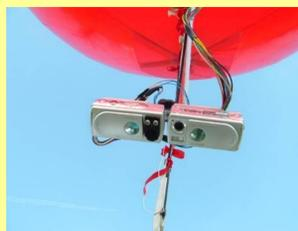
Fig. 3. Two Sony DSC-U30 digital camera payload of the Helikite.
